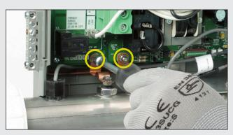
Use a 3/8" (9.5mm) nut drive to remove the 2 nuts on the circuit board holding the heater copper straps to the system.
